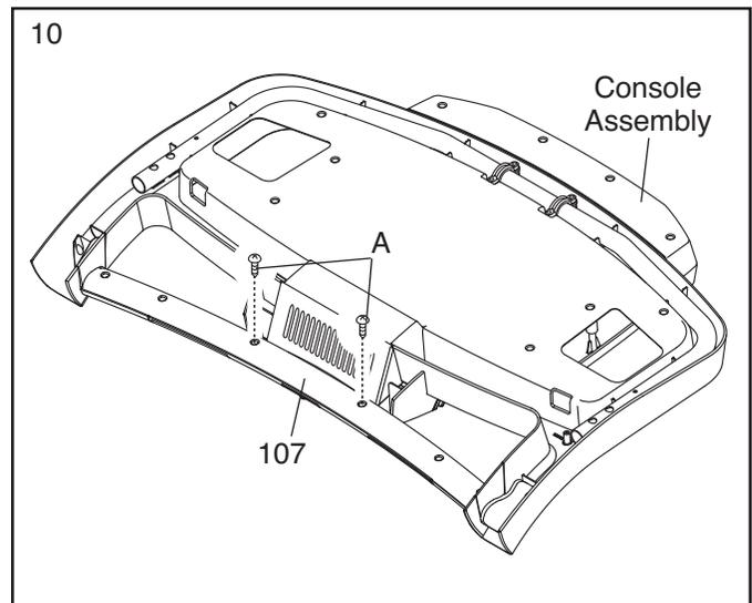
11. **IMPORTANT: To avoid damaging the Crossbar (107), do not use power tools and do not overtighten the #10 x 3/4" Screws (4) or the #10 x 3/4" Flat Head Screws (109).**
