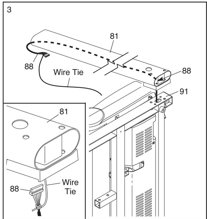
4. Hold the Right Upright (81) against the Base (91). **Be careful not to pinch the Upright Wire (88).** Insert two 3/8" x 4" Bolts (7) and a 3/8" x 1 1/2" Bolt (8) with three 3/8" Star Washers (11) into the Right Upright.
