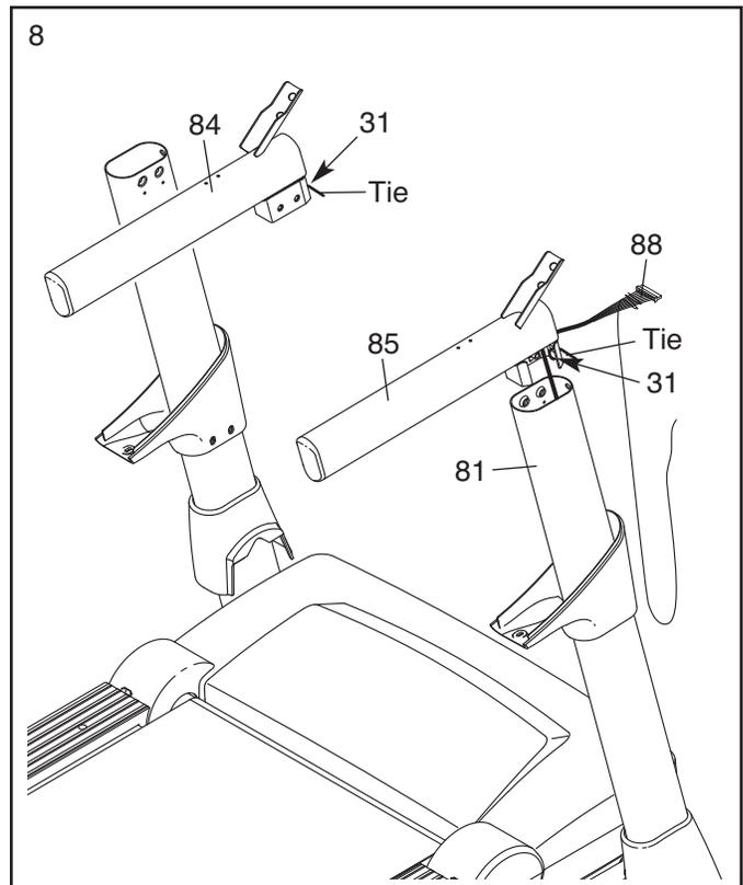
9. Attach the Right Handrail (85) to the Right Upright (81) with two 5/16" x 1" Bolts (5), two 5/16" Star Washers (13), and a 5/16" x 1 1/4" Bolt (2). **Do not fully tighten the Bolts yet.**
