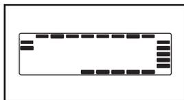
**The left display**—The left display will show the elapsed time, the incline of treadmill, and the approximate number of calories you have burned for a few seconds each. Press the left Display button until the display shows the information that you are most interested in viewing. Note: When some workouts are selected, the display will show the time remaining in the workout instead of the elapsed time.
