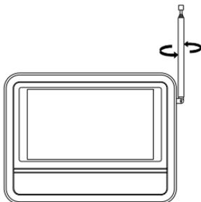
**Removing Direct-Connect Antenna** Before connecting a different antenna or a coaxial cable, you need to remove the direct-connect antenna first.
