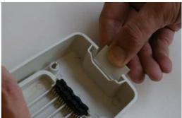
Now connect the cables from the turntable on the cables from the interior of the vehicle, within the casing (see illustration on the right).
