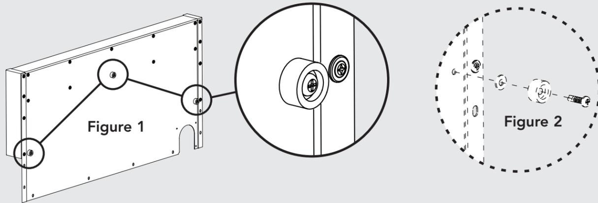
Simply slide the backguard down onto the rear of the unit until it settles on the shoulder screws located on the back of the range.
