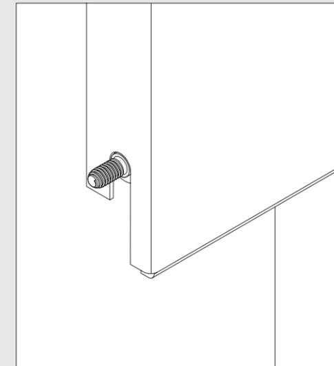
Once the high-shelf back is in position, attach using the (4) screws provided. Once secured to the range, place the top rolled edge (X) of the high shelf over the front lip of the high-shelf back.
