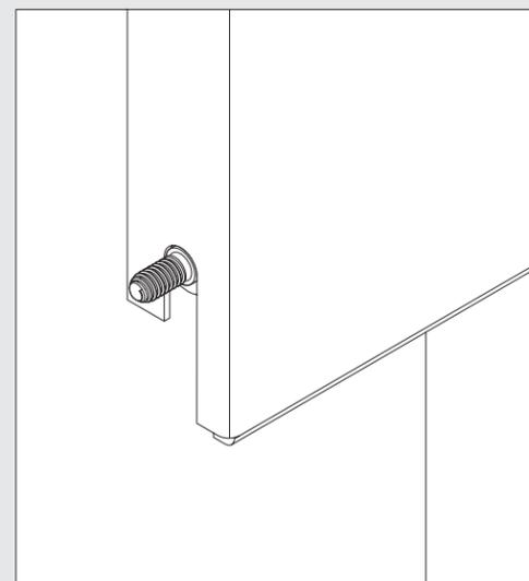
Once the backguard is in position, attach using the (4) screws provided.
