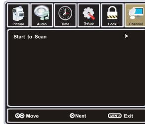
If you select "Air" as input signal in Antenna item, you can press RIGHT button to search the channels automatically.
