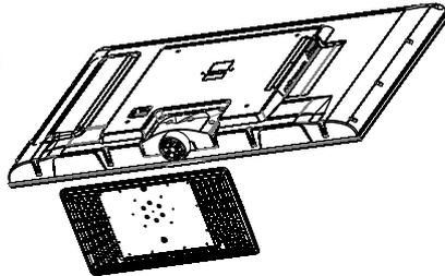
2. Fix the base cover to fixed-ring base with the screws.
