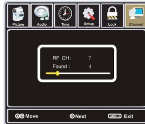
If you select "Cable" as input signal in Antenna item, allows you to select Cable System among: AUTO, STD, IRC and HRC. Use DOWN button to highlight the "Start to Scan", then press RIGHT button to search the channels automatically. The receivable channels will be stored automatically. When searching channels, press MENU to stop.
