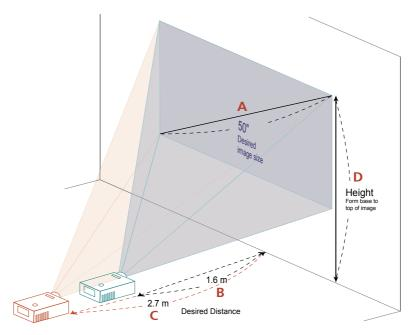
The table below shows how to achieve a desired image size by adjusting either the position or the zoom ring. For example: to obtain an image size of 50" set the projector at a distance 1.6 m and 2.7 m from the screen and adjust the zoom level accordingly.
