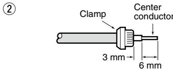
Strip the cable and fold the braid back over the clamp.
