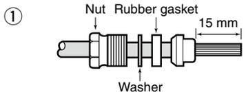
Slide the nut, flat washer, rubber gasket and clamp over the coaxial cable, then cut the end of the cable evenly.
