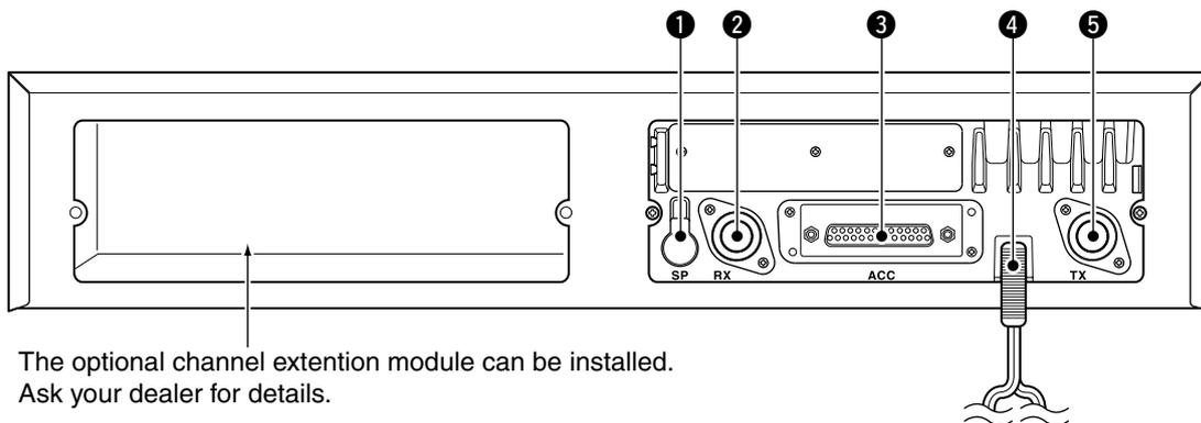
The optional channel extension module can be installed. Ask your dealer for details.
