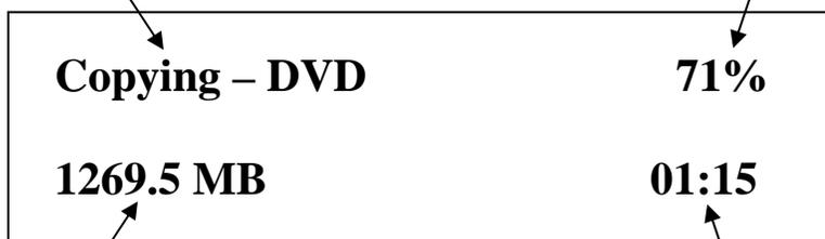
Displays the amount of data left to be recorded. This number starts at the capacity of the master and counts down.
