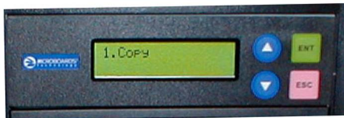
ENT button: The ENT button, used to start a duplication process or enter into an area in the menu structure.
