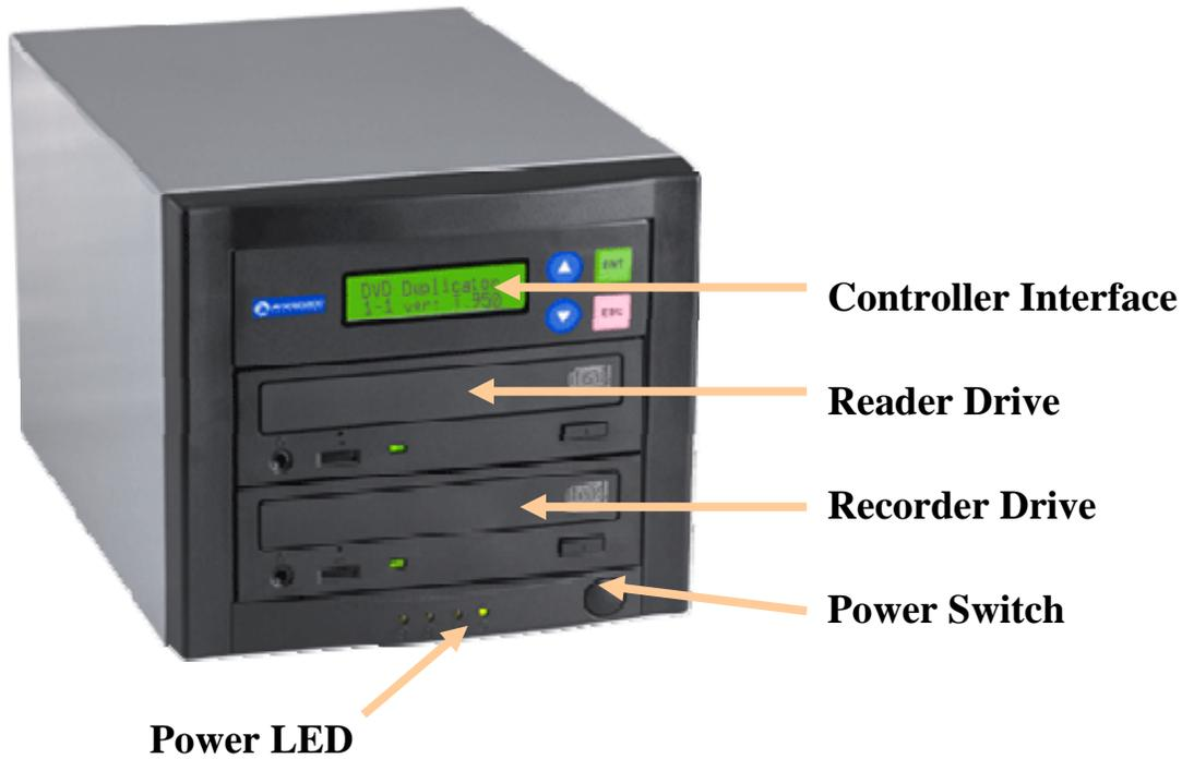
The QD-DVD system consists of a DVD reader, DVD Writer, USB Connection, and Controller module.
