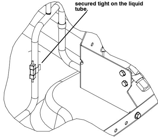
Fig. 9 - Outdoor Coil Thermistor (OCT) Attachment
