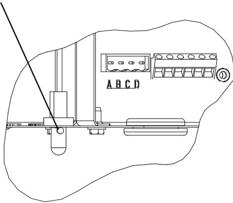
Fig. 8 - Outdoor Air Thermistor (OAT) Attachment
