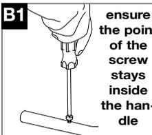
ensure the point of the screw stays inside the handle
