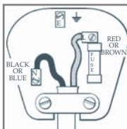
The wires in the mains lead are coloured in accordance with the following code:
