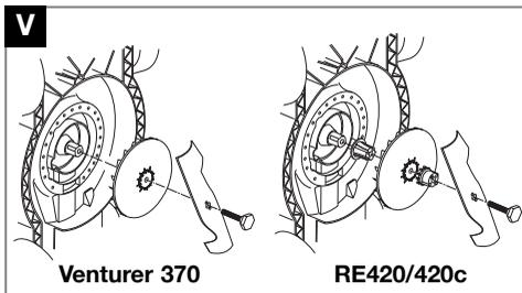
**Always handle the blade with care - sharp edges could cause injury. USE GLOVES. Renew your metal blade after 50 hours mowing or 2 years whichever is the sooner - regardless of condition. If the blade is cracked or damaged replace it with a new one. Never use a blade bolt if the insulated head is damaged cracked or missing.**
