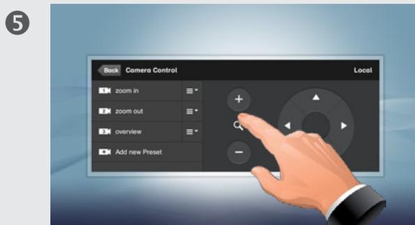
Use **+** and **-** to adjust the zoom and the arrow keys to adjust the camera's angle. You may also define or edit camera presets in this menu, see ► "Adding a near end camera preset" on page 6 for details.
