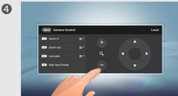
Entering **Camera Control** will also cause the system to show selfview, so if you know that camera adjustments are needed, you do not have to activate selfview first.
