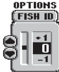
Decreasing the value to a number less than zero shows fewer fish symbols on-screen. In this case smaller sonar returns are disregarded. This is useful for eliminating many small sonar returns when seeking larger species of fish.
