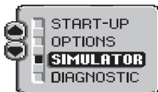
When in simulator operation, the **425SX** responds to control inputs as if it is in actual operation, so feel free to experiment, or to customize the unit for your particular operation.
