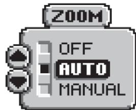
“Automatic” Zoom is especially helpful when looking for structure or bottom detail. The “Automatic” Zoom keeps the bottom in view even in quickly changing terrain. “Manual” Zoom provides detailed information of any area from the surface to the bottom.
