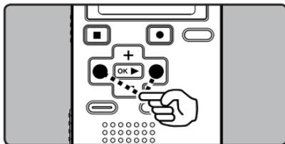
While the recorder is during stop mode or playback mode, press the **▶▶▶** button.
