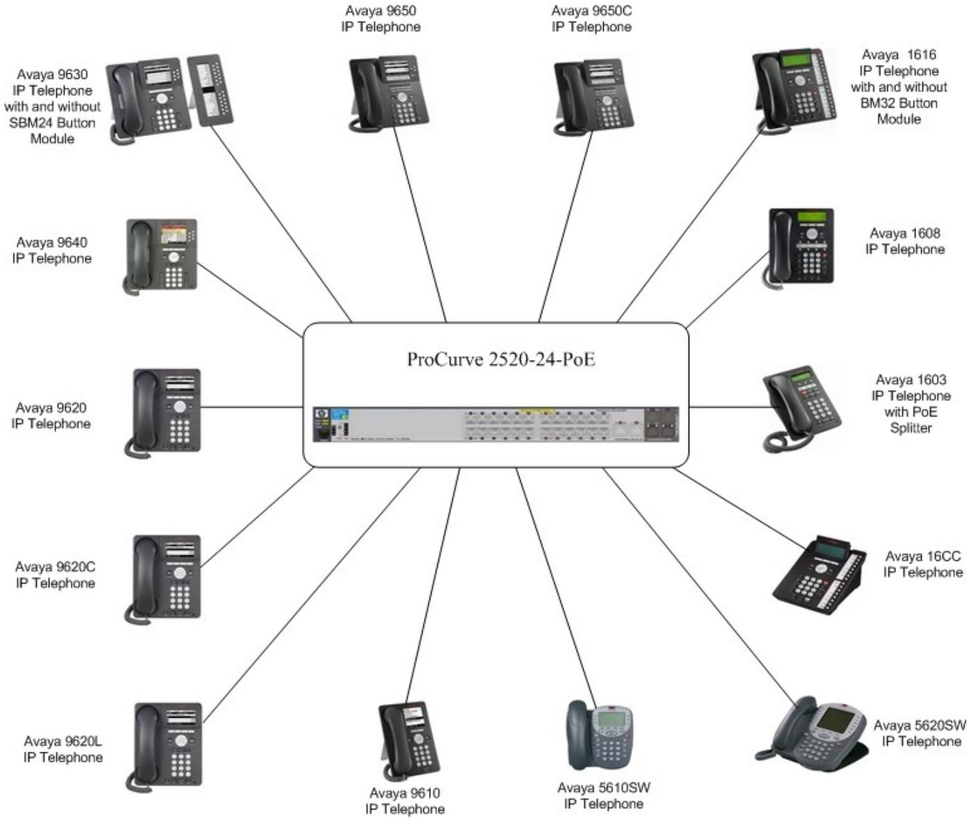
**Figure 1: HP ProCurve 2520-24-PoE Switch and Avaya IP Telephones**
