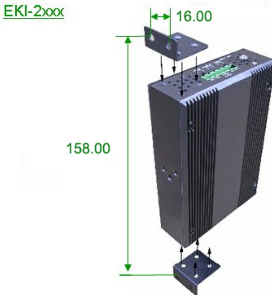
Figure 2.5: Combine the Metal Mounting Kit (units: mm)
