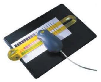
If the Spectrocam was not previously calibrated, a prompt directs you to calibrate the white reference. Place the measurement device on the white target reference and touch the green sensor to calibrate. After calibrating with the white reference, reposition the measurement device on the first patch on the upper, left corner of the test form.
