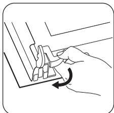
**5** Release the locking system to remove the panels of glass.
