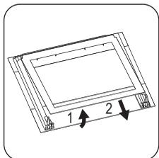
**7** Carefully lift (step 1) and remove (step 2) the panels of glass one by one. Start from the top panel of glass.
