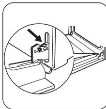
**1** Open the door fully and hold the two door hinges.
