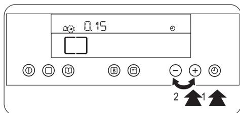
1. Set an oven function and a temperature (not necessary for the Minute Minder). Refer to "Setting the oven function".
