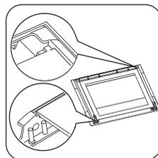
Make sure that you install the top panel of glass in the seats correctly.
