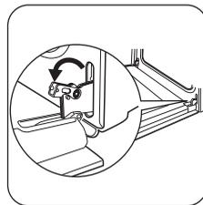
**2** Lift and turn the levers on the two hinges.
