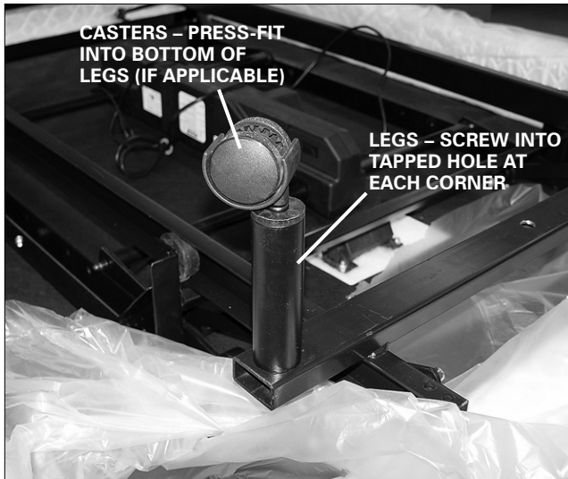
FIGURE 1: Precision Comfort™ leg installation. Caster installation (if applicable).
