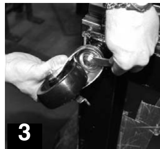
3 Use the tool provided to tighten the castor into place.
