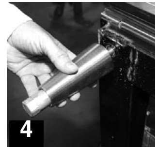
4 Thread leg into cabinet bottom frame rail.
