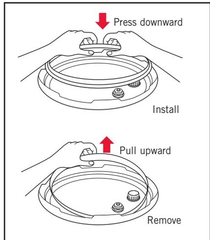
Figure 1. Removing and reaffixing the sealing gasket.
