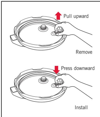
Figure 2. Clearing the steam release valve cover.
