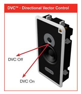
By flipping the DVC switch to "on," we electronically manipulate the crossover so that the speaker's midrange output lobes down about 15 degrees from the speaker. This is perfect for when this speaker is mounted above ear level and you want to
