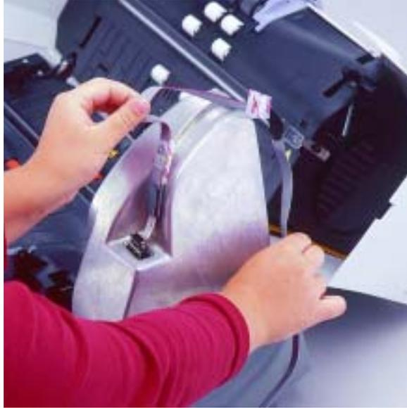
13. Peel off the backing from the first self-stick hook-and-loop pad that is attached to the imprinter cable.
