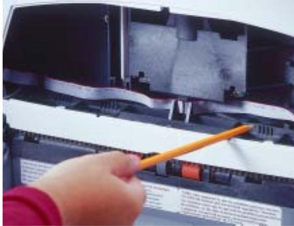
6. Lift the ink cartridge carrier out of its position.
