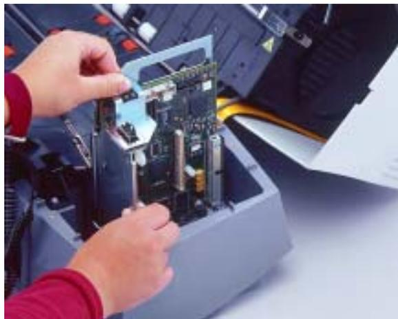
6. Attach and tighten the fourth thumbscrew on top of the circuit board mounting bracket.
