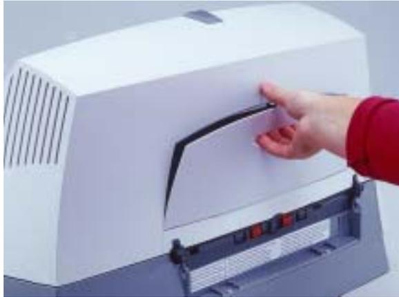
3. Lift the imprinter access door off the scanner.
