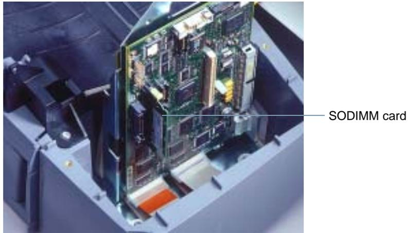
12. Plug the new SODIMM card into the main control board.
