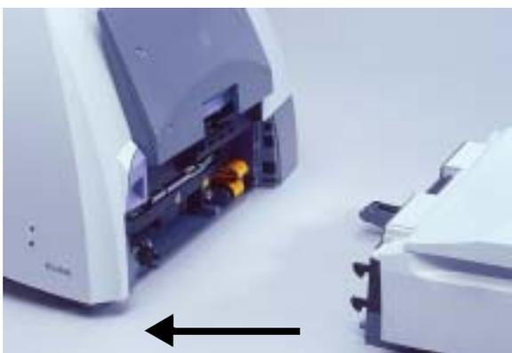
6. Push the flatbed against the scanner until the docking latches click into place.
