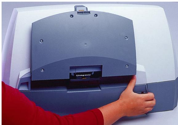
4. Remove the scanner front panel.
