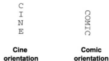
The resolution of the character fonts is 96 dpi across the width of the scanner. However, the font resolution varies with the direction that the paper is fed into the scanner. This variable allows the creation of an easy-to-read character string. The approximate resolution of the printed output is shown below.
