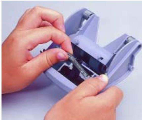
7. Re-install the separator module and align the shaft ends.
