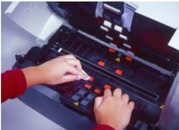
2. Clean any dust or debris in the slots around the drive rollers.
