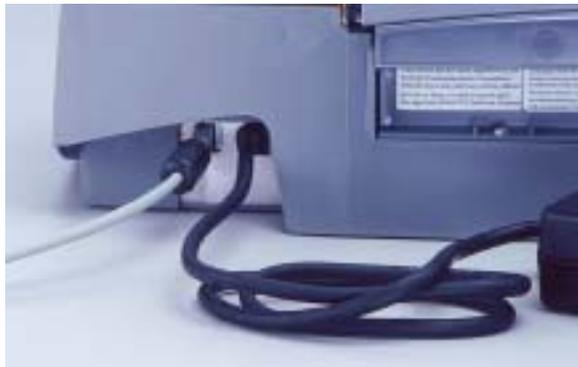
4. Disconnect the IEEE-1394 (FireWire) cable from the IEEE-1394 port on the back of the scanner.
