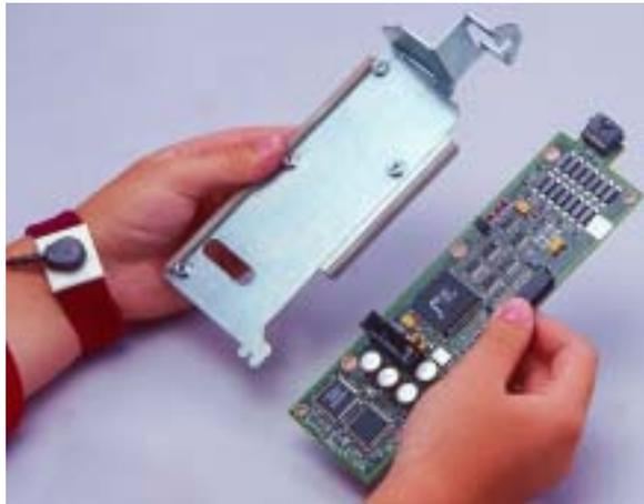
2. Align the three thumbscrews on the imprinter board with the corresponding holes on the circuit board mounting bracket.
