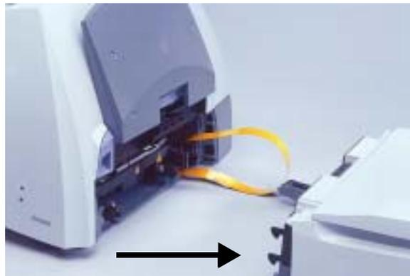
5. Remove the scanner front panel from its storage place on the back of the flatbed.
