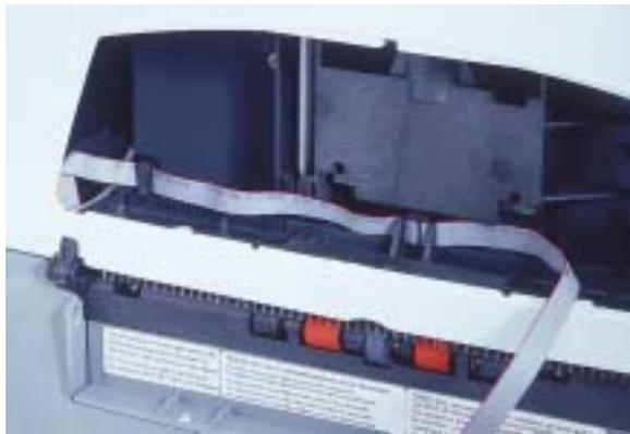
This assures that the imprinter cable will not be pulled too tightly when the scanner door is opened.
