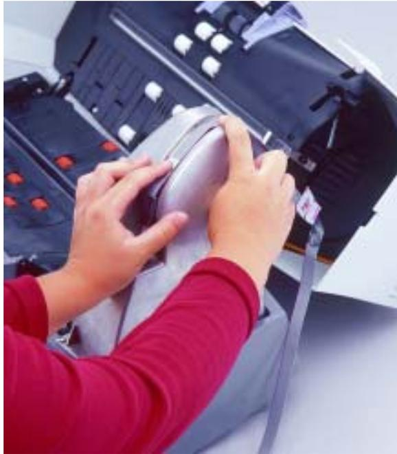
15. Continue to align the imprinter cable along the channel in the circuit board cover until it is behind the circuit board cover.
