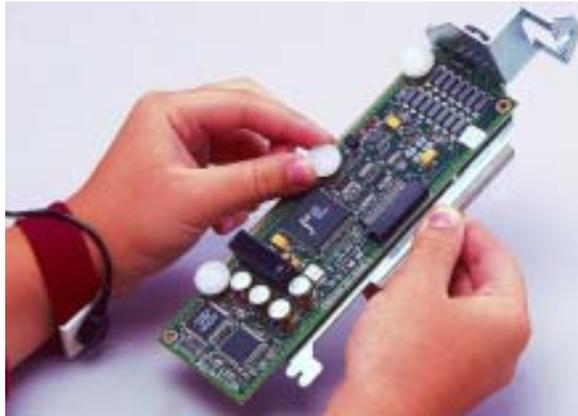
4. Slide the hook near the bottom of the circuit board mounting bracket into the support slot on the main control board.
