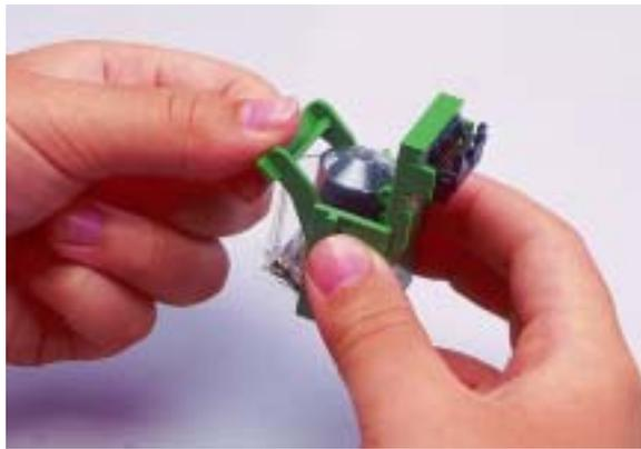
9. Slide the ink cartridge carrier into its position.
