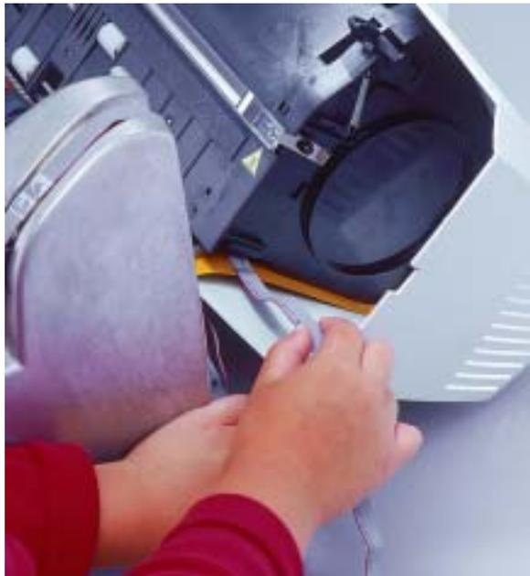
19. Lower the scanner door and press it down firmly until it latches into place.
