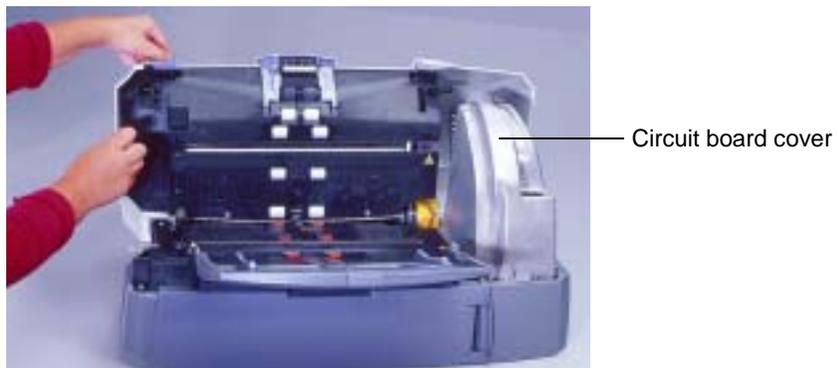
8. Use a Phillips-head screwdriver to remove the two screws (one front, one back) that hold the circuit board cover in place.
