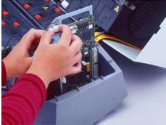
7. Make sure that the imprinter board is seated and secure.
