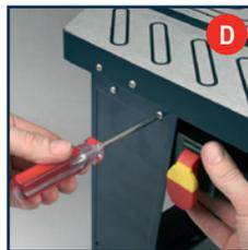
6. Secure the switch box to the leg with the 2 Philips head screws (fig. D).
