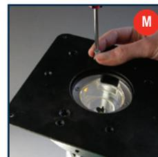
4. Secure the router plate to the table by feeding each of the 4 screws through the top of the table and into the router plate (fig. N).
