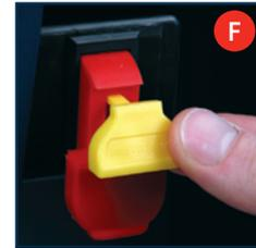
**Note.** The on/off switch features a switch disabling insert for greater safety when the tool is left unattended. The switch disabling insert must be in place before using the tool (fig. F).
