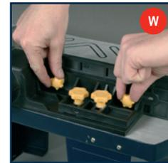
1. To slide the fence backwards and forwards loosen the two fence locking knobs (fig. T). This will set the infeed fence (9) to support the workpiece (fig. U).
