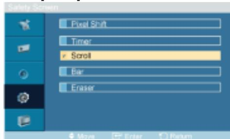
This function prevents after-images on the screen by moving all the pixels on the LCD according to a pattern.
