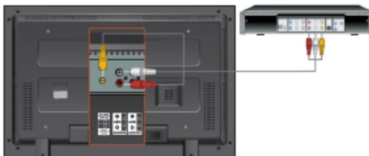
1. Connect the port of the DVD, VCR (DVD / DTV Set-Top Box) to the [R-AUDIO-L] port of the LCD Display.
