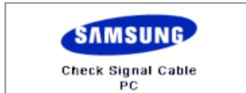
4. Turn off your LCD Display and reconnect the video cable; then turn on both your computer and the LCD Display
