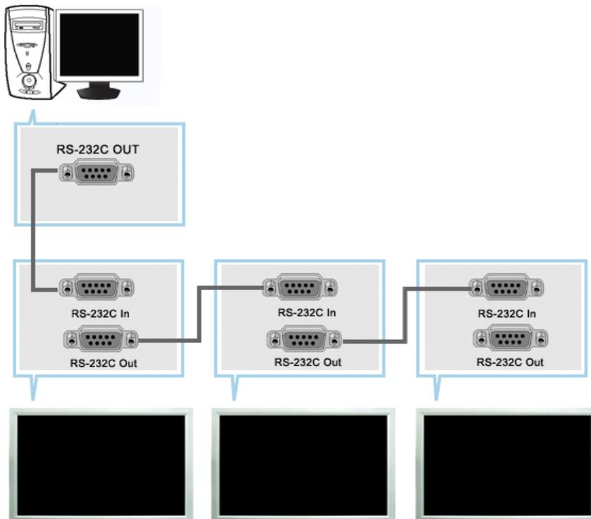
A Multiple Display Control (MDC) is an application allowing various displays to be easily and simultaneously operated on a PC. RS-232C, a standard of serial communication, is used for the communication between a PC and a display. Therefore, a serial cable should be connected between the serial port on a PC and the serial port on a display.
