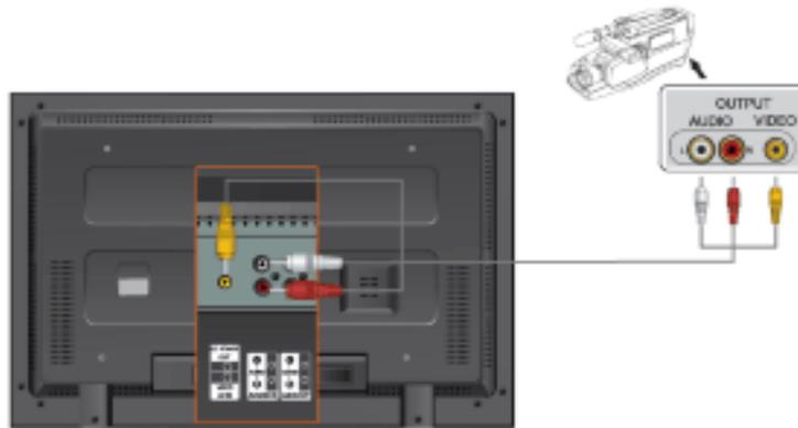
1. Locate the AV output jacks on the camcorder. They are usually found on the side or back of the camcorder. Connect a set of audio cables between the AUDIO OUTPUT jacks on the camcorder and the AV AUDIO IN [L-AUDIO-R] on the LCD Display .
