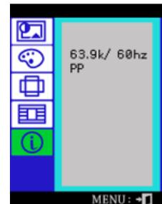
You can see the frequency (user control mode) used by the user, the polarity of the operational signals, the default frequency (default mode) set when you buy the monitor and the resolution level.
