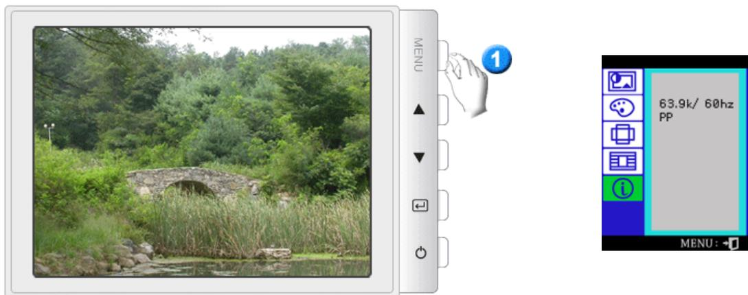
You can see the frequency (user control mode) used by the user, the polarity of the operational signals, the default frequency (default mode) set when you buy the monitor and the resolution level.
