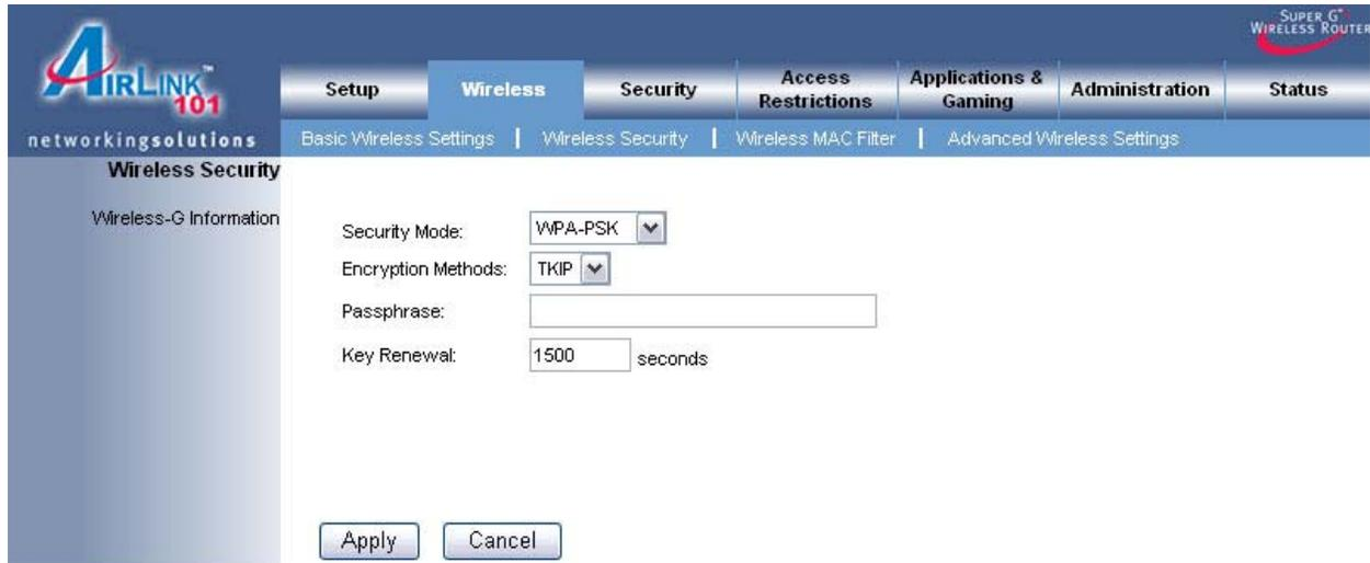
The screenshot shows the configuration interface for a Super G Wireless Router. The top navigation bar includes tabs for Setup, Wireless, Security, Access Restrictions, Applications & Gaming, Administration, and Status. The 'Wireless' tab is active, and the 'Wireless Security' sub-tab is selected. The main content area is titled 'Wireless Security' and contains the following settings:
