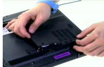
6. Remove the four screws holding the thermal module. (Follow the order indicated by the numbers: 4, 3, 2 then 1. Please reverse the order when you assemble the system).
