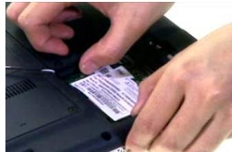
5. Remove the two screws fastening the HDD cover.
