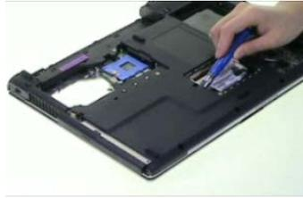
3. Open the LCD module as shown and detach the middle cover carefully.
