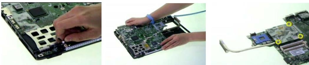
6. Disconnect the VGA board assembly from the main board.
