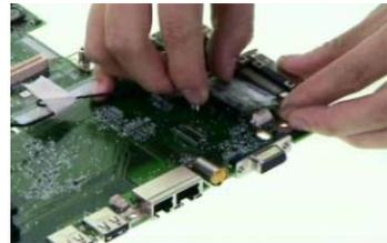
12. Disconnect the modem cable from the modem board.
