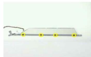
10. Then remove the LCD right bracket.
