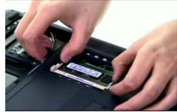
4. Remove the two screws fastening the thermal door.
