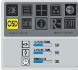
This changes the position of the OSD window on the screen. TIMEOUT function allow user define the OSD appearing period from 10 seconds to 60 seconds.
