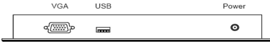
15-pin D-sub VGA and USB-type touch screen
