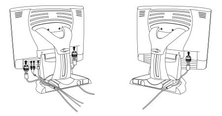
Once you have connected your M150 FPD monitor to your computer, you should take advantage of the cable management system designed into the base of the M150 FPD monitor as shown above.
