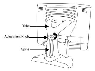
The newly redesigned M150 monitor features an innovative design adjustable to approximately 60° off the vertical to accommodate different counter and user heights, a positive locking mechanism, a weighted base for additional stability, a touch screen interface, several mounting options, and built-in cable management.
