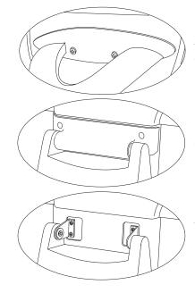
Figure 1 Disassembling the Yoke & Base for Arm Mounting
