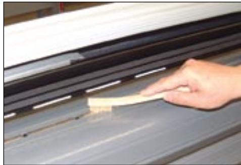
Figure 27. Cleaning the Drive Shaft.
