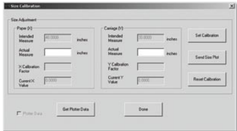
Figure 29. Calibration screen in Control Center .
