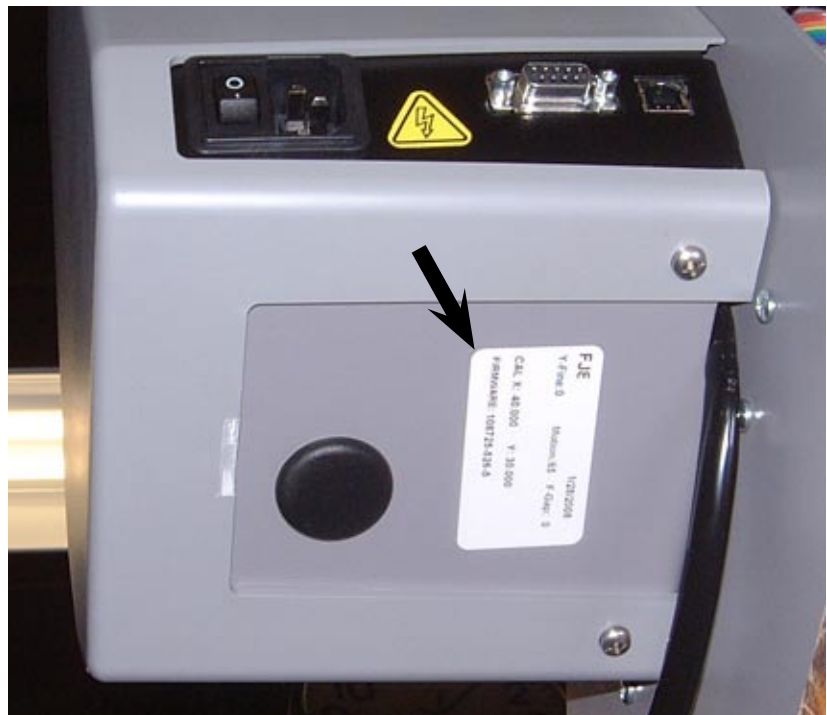
Figure 35. Factory calibration values on the sticker under the right end cover.
