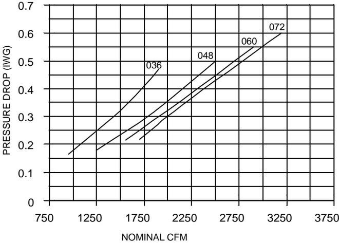
**FIG. 15 PRESSURE DROP vs SUPPLY AIR CFM**
