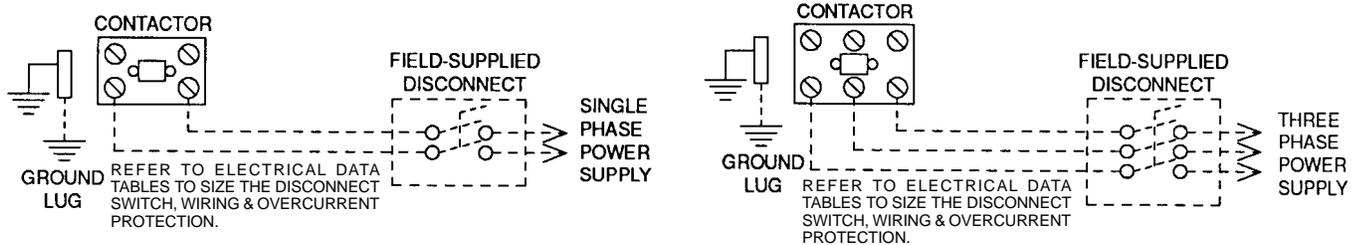
**FIG. 2 - TYPICAL FIELD WIRING**
