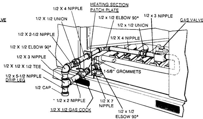
**FIG. 4 - BOTTOM SUPPLY CONNECTION
