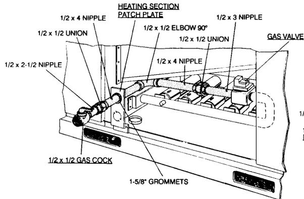
**FIG. 3 - EXTERNAL SUPPLY CONNECTION
