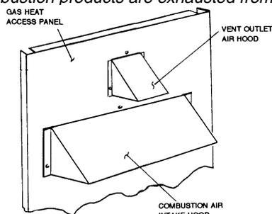
**FIG. 5 - VENT AND COMBUSTION AIR HOODS**
