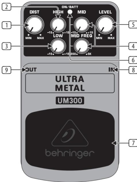
1 The **LOW** control allows you to boost/cut the lo-frequency range.
