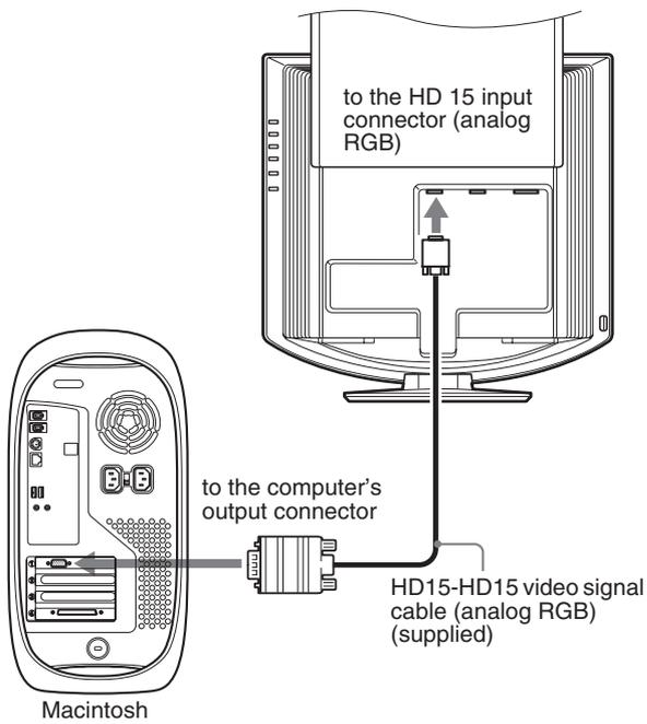
When connecting a Macintosh computer, use an adapter (not supplied), if necessary. Connect the adapter to the computer before connecting the video signal cable.
