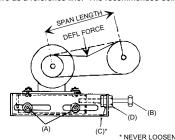
Tension new belts at the max. deflection force recommended for the belt
