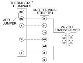
24 VOLT THERMOSTAT 2TH07701024. IF THE UNIT HAS AN ECONOMIZER, REMOVE JUMPER J1 FROM TERMINALS 8 AND 10 ON THE RELAY BOARD TO PREVENT SIMULTANEOUS OPERATION OF THE SCROLL COMPRESSOR AND THE ECONOMIZER. IF YOU WANT TO CONTROL THE ECONOMIZER ON A SECOND STAGES OF COLING OR HAVE AN ELECTRIC HEAT ACCESSORY WITH TWO STAGES OF HEAT, USE THERMOSTAT 2TH04701024.
