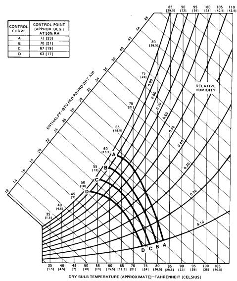
FIG. 7 - ENTHALPY SET POINT ADJUSTMENT
