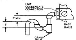
FIG. 1 - RECOMMENDED DRAIN PIPING
