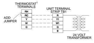
COOLING / HEATING (24 VOLT ELECTRONIC THERMOSTAT)
