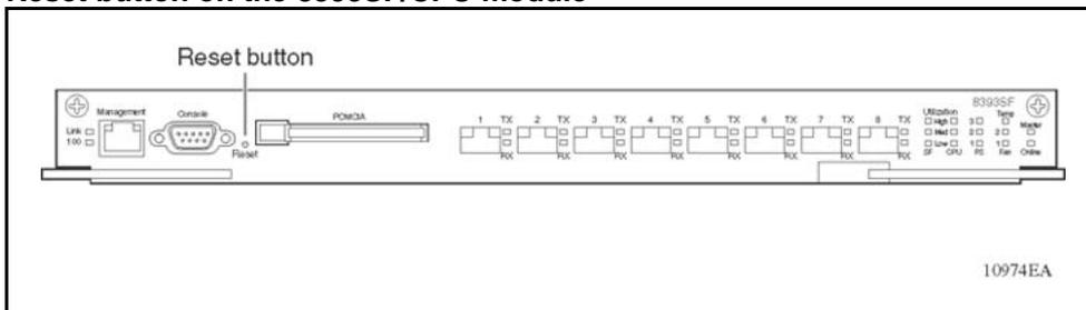
The following figure shows the location of the Reset button on the Ethernet Routing Switch 8394SF/CPU module.
