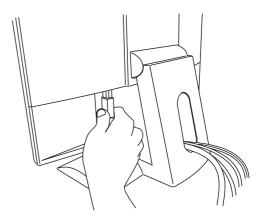
4. Connect the other end of signal cable to the signal connector of your computer. Connect audio cable to your computer.
