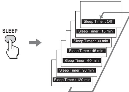
While Sleep Timer is activated, the PIC OFF/TIMER LED on the unit lights up in orange.
