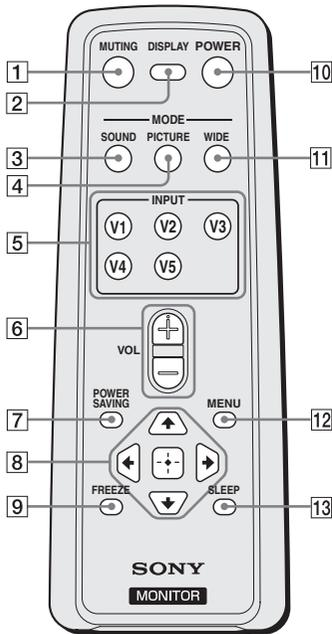
The VOL + button has a tactile dot. Use it as a reference when operating the unit.
