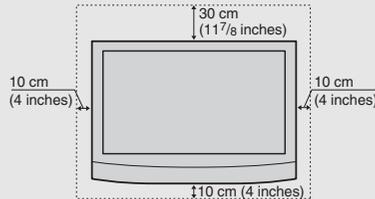
When installing the unit using a stand, allow this much space.
