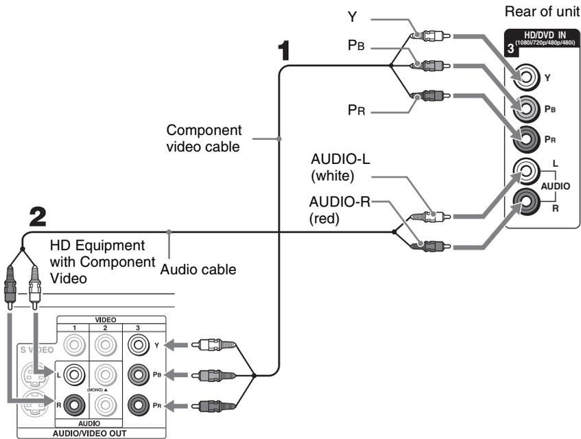
✍ Some of the HD equipment you can connect to receive the broadcasting signals are digital cable box, digital satellite receiver and digital TV receiver.
