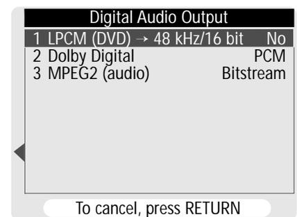
\* Does the DVD contain an audio format of higher quality than 48kHz/16bit (maybe 96kHz/24bit), the player has to convert into a format compatible to DAT or MD. Switch back to "No", to hear via your sound system the better sound quality possibly recorded to a DVD.
