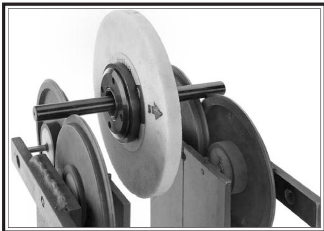
**Figure 39. Wheel on balancing fixture.**
