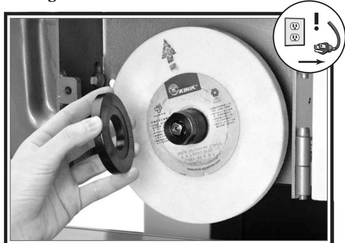
Figure 25. Wheel ready for removal.
