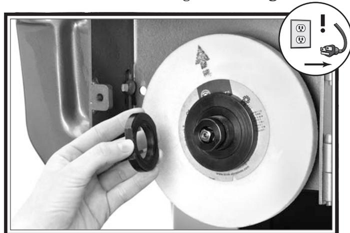
Figure 24. Exposing wheel retaining washer.
