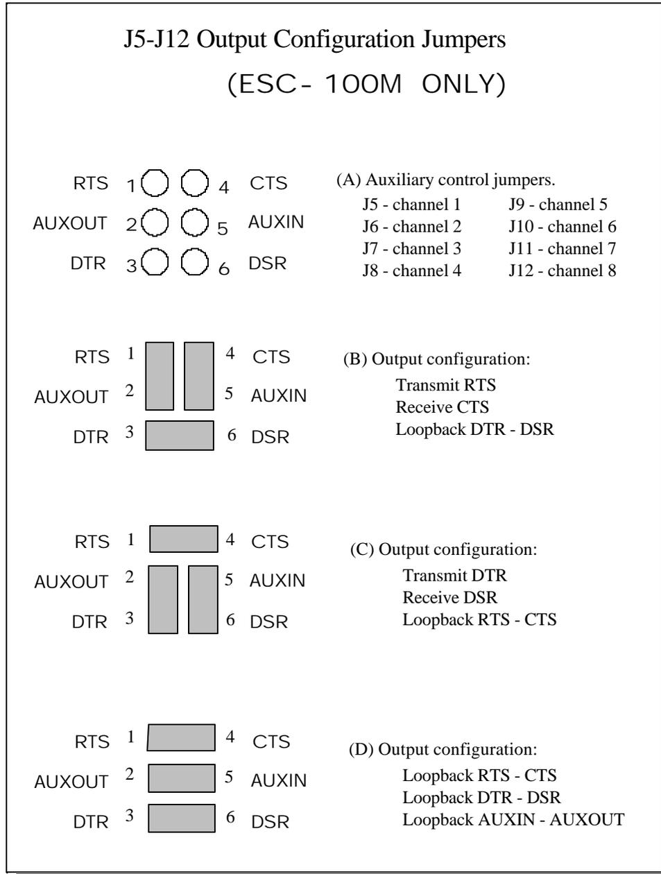
Figure 22 --- ESC-100M Auxiliary Signal Configuration Jumpers
