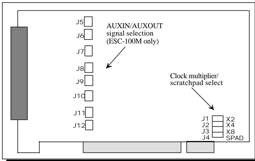
Figure 5 --- Jumper/connector locations
