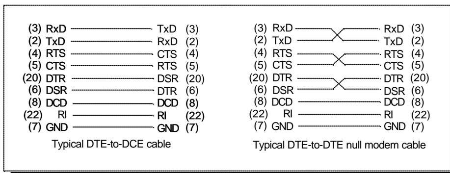
Figure 17 --- Cabling requirements for RS-232-C devices
