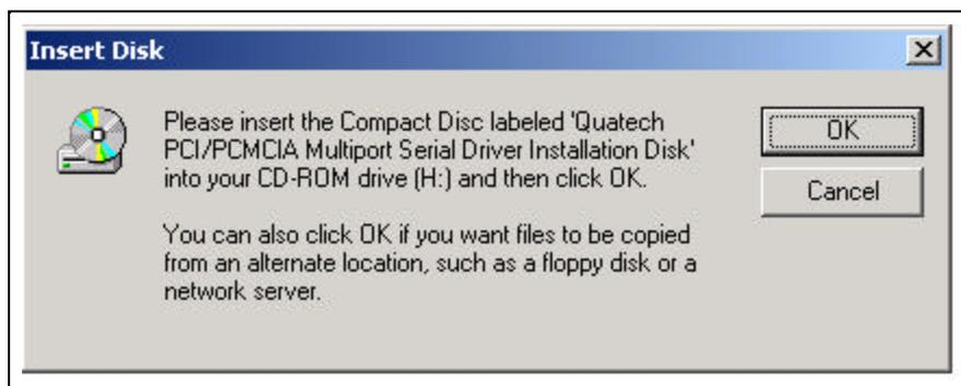
2. The following dialog box insert the Quatech COM CD (shipped with the device). Click the "OK" button.
