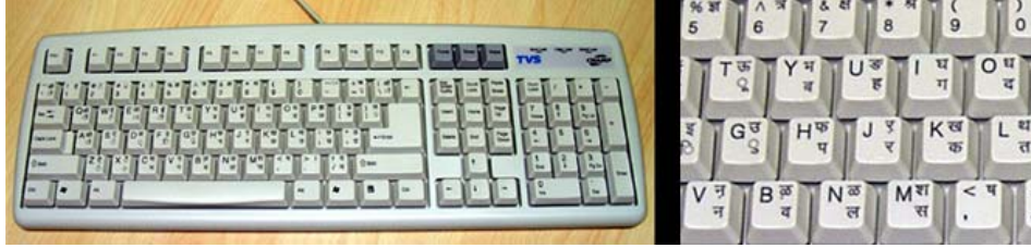
Figure 2: Inscript keyboard (with multiple characters on a single key)
