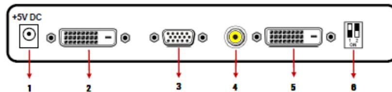
*To reset the DVI-SPLITPRO-2B to factory default settings: Turn on the DVI-SPLITPRO-2B then switch both DIP Switches simultaneously up and down to reset the unit to factory default settings*
