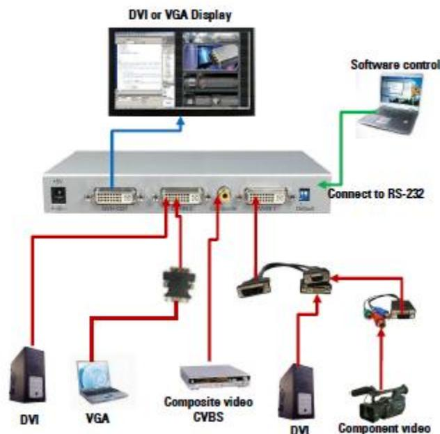
8. Connect a device equipped with composite video output to composite input of the DVI-SPLITPRO-2B.
