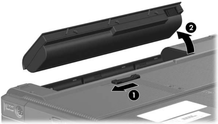
Removing the Battery Pack
