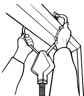
Check that clamp is secure on door frame by pulling firmly down on the clamp cover. If molding moves, repair it before using the jumper.
