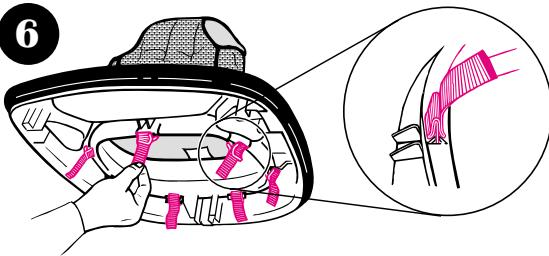
Pull the 7 short straps through the slots until the loops are completely through the slots. The two loops on the short straps must overlap edges of the slots as shown.
