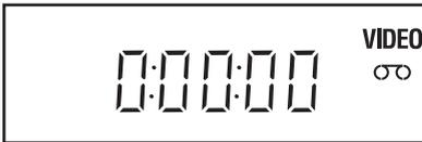
To display the counter on the TV screen, press DISPLAY during normal playback.
