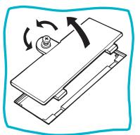
Insert 4 x 1.5V "AA" or LR6 batteries according to the diagram on the inside of the battery compartment.
