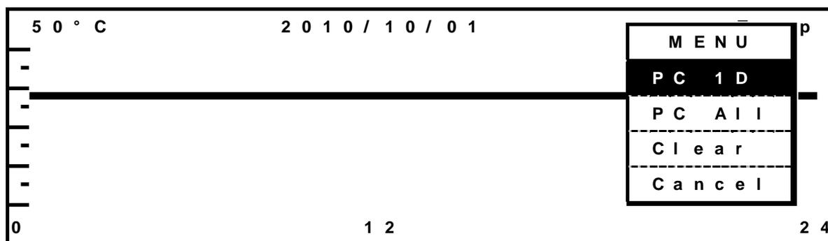
2. A Progress Display will appear. On a HyperTerminal on PC, specify a transfer, text capture, and the name of the file to save. Use TXT or CSY as the file name extension. Press the MENU Key to display the menu, select **Start**, and press the ENTER Key.
