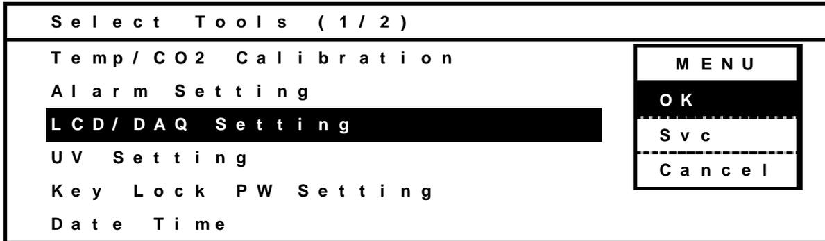
2. The LCD/DAQ Setting Display will appear. Set the initial setting for each parameter as necessary.
