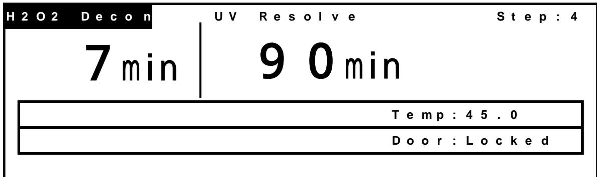
9. After completion of H<sub>2</sub>O<sub>2</sub> mist generation, “UV Resolve” will flash at the top of the screen, and H<sub>2</sub>O<sub>2</sub> gas resolution by UV light will start.
