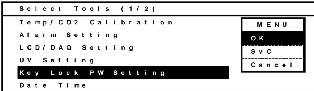
3. Input the current user password (4 digits), select **OK**, and press the ENTER Key. (The default user password is 0000 when the Incubator is shipped from the factory.)
