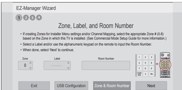
1. Complete the appropriate field(s) as described below. Use the Left/Right arrow keys on the Installer Remote to navigate between each of the fields.
