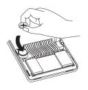
Snap the front and back case halves back together, then replace the screws.
