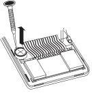
Position the new battery so the positive (+) side is up, then insert it into the battery compartment.
